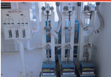
Sulfide Stress Corrosion Cracking Tester (SSCC)
