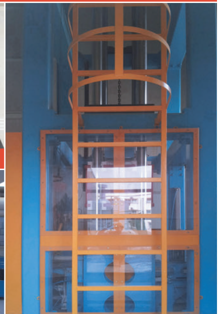
Drop Weight Tear Tester (DWTT)
