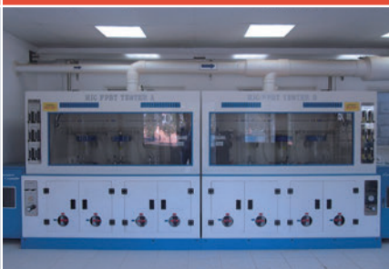
Hydrogen Induced Cracking Tester (HIC)
